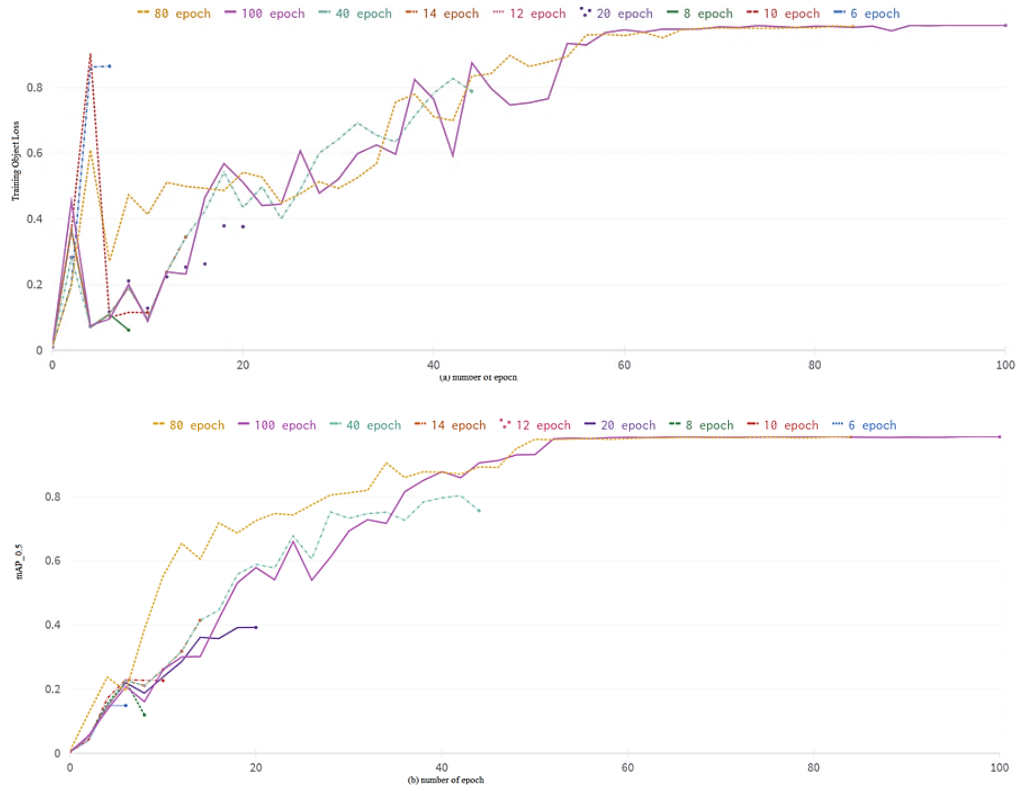
Figure 3. Accuracy performance as the number of epochs is increased (a) precision and (b) mAP
