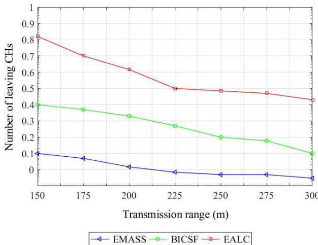
FIGURE 9. Number of CHs leaving the cluster vs transmission range.
