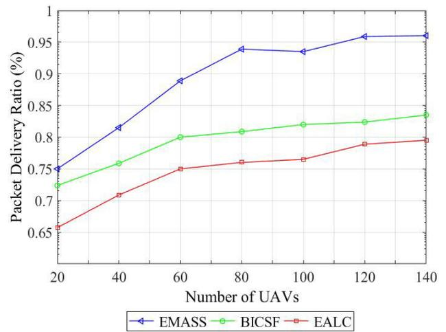
FIGURE 7. PDR for different densities of UAVs.
