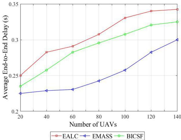
FIGURE 8. Average EED for different densities of UAVs.
