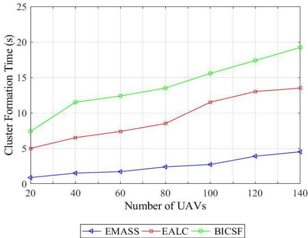
FIGURE 4. Cluster formation time required for different densities of UAVs.
