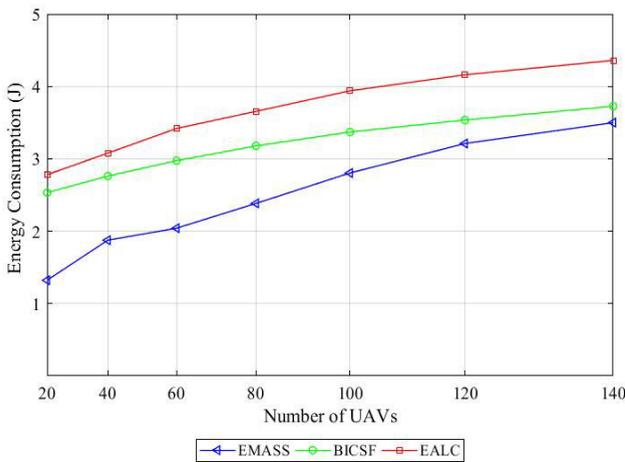
FIGURE 5. Energy consumption for different densities of UAVs.
